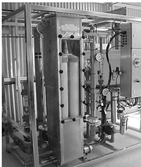
Figure 3: The PVP used to test the effect of Waranga water on Membrane filtration
