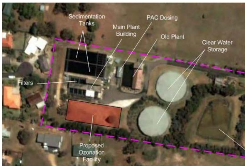
**Figure 1:** *Site Plan Showing Location of Proposed Facility*
