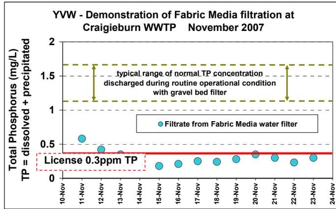
filtrate. The resolution required a tenfold pre dilution of the alum and higher dose pump speed providing consistent coagulation of the raw water.
