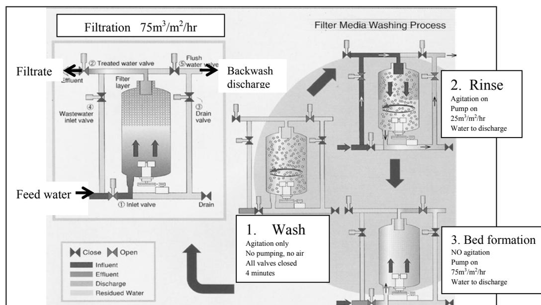
**Figure 2:** The backwash cycle
