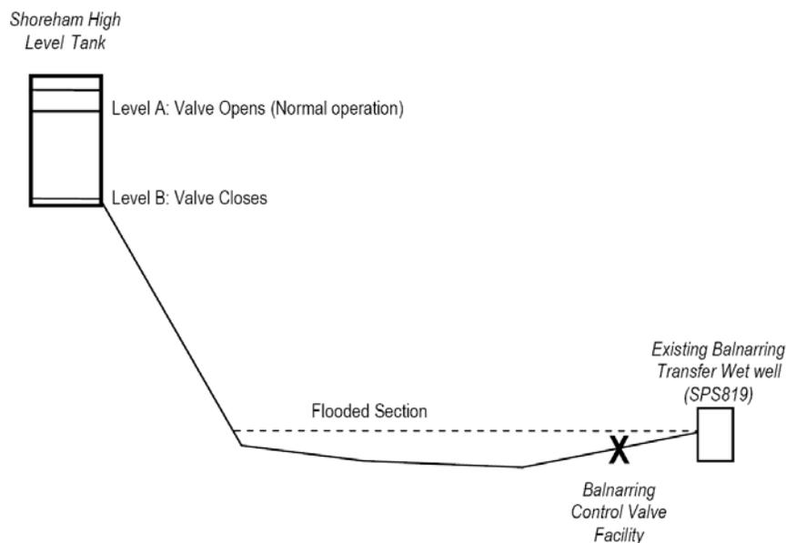
**Figure 4:** *Shoreham High Level Tank to Balnarring - Control System Schematic*
