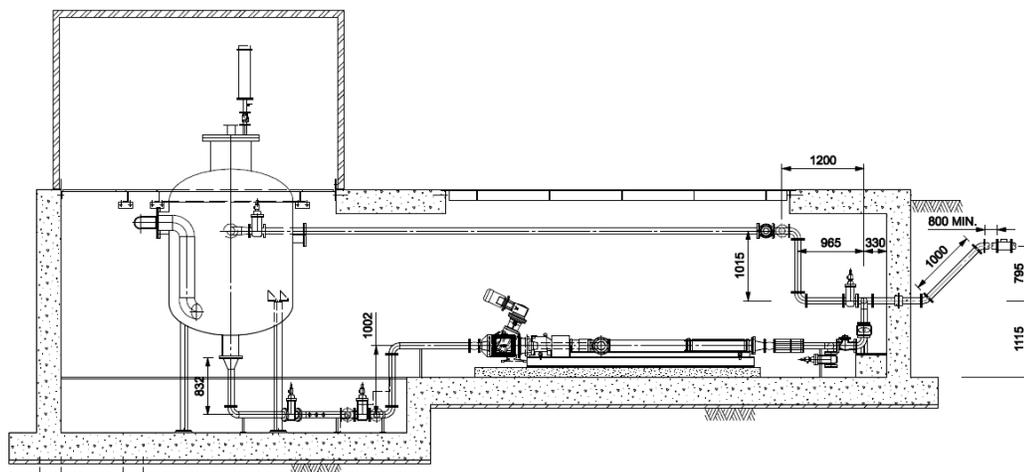
**Figure 3:** *Cross-section plan of the Pressure Sewer Pump Station concept*
