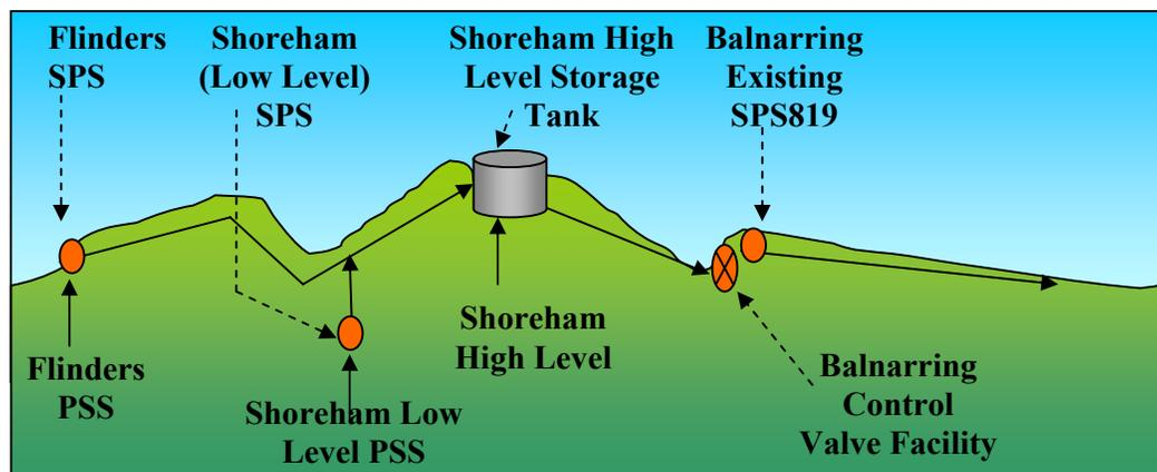
**Figure 1:** *Schematic of the Flinders/Shoreham Sewerage Transfer System*
