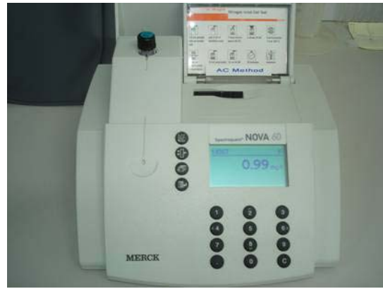
Figure 3: Alzarin complexone spectrophotometer - secondary/backup system
