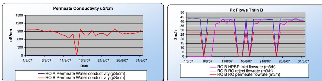
**Figure 6:** *Typical permeate water conductivity and recovery reports from data transfer – KSC, Hong Kong*
