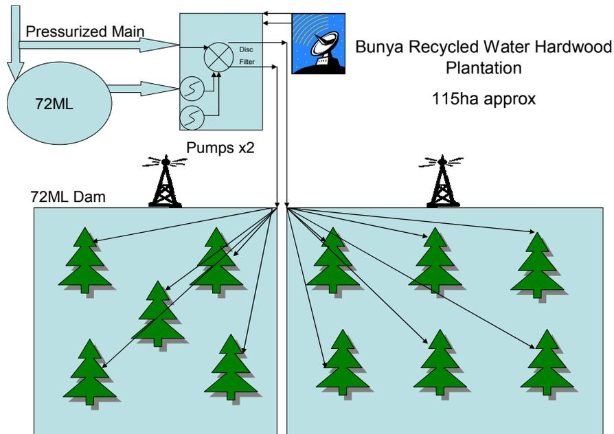
**Figure 6:** Bunya Farm irrigation layout Schematic
