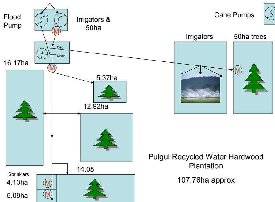
**Figure 1:** Schematic of the Pulgul Irrigation Area
