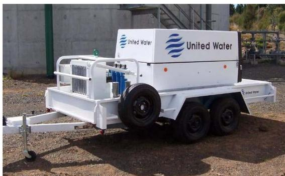
**Figure 3: Trailer Mounted Air Scouring Unit**
