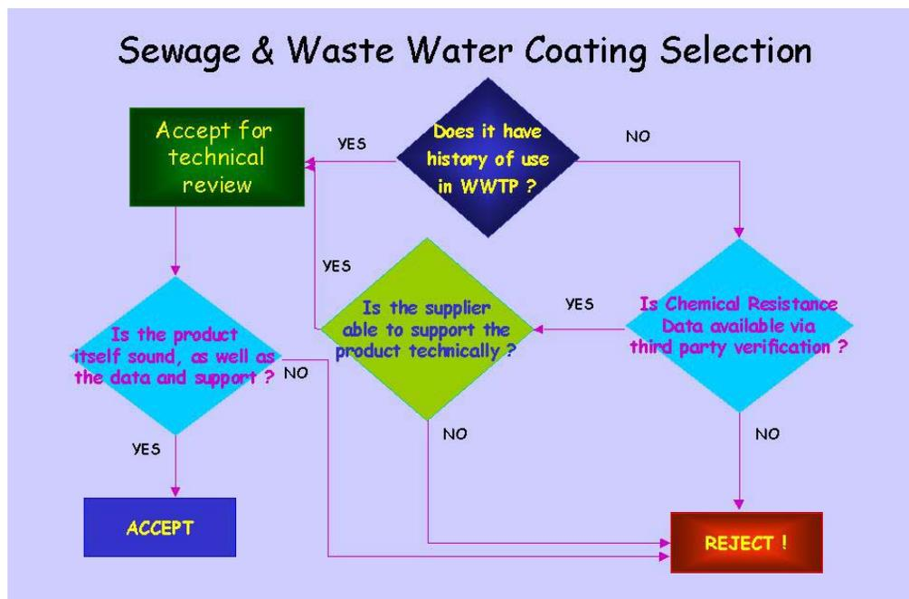
**2.6** **Figure 1:** *Flowchart for Sewage & Wastewater Coating Selection*
