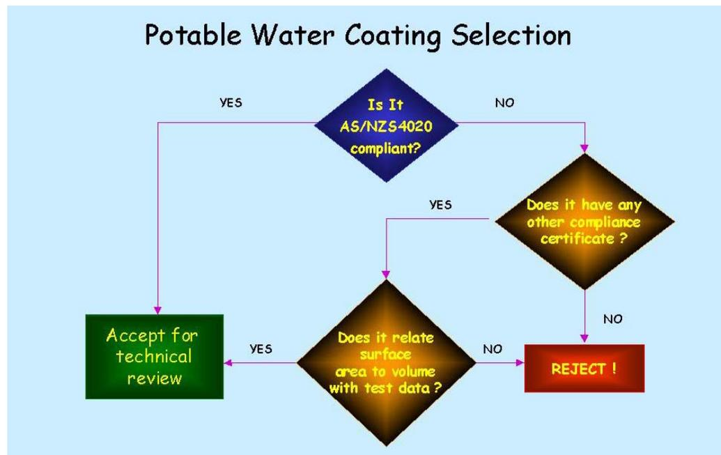
**Figure 2: Flowchart for Potable Water Coating Selection**
