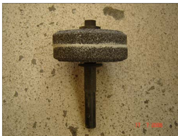
Figure 1: Photograph of a PCDM nozzle and stem
