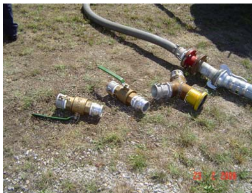
Figure 2: Fittings for submersible pump, including "y" junction.
