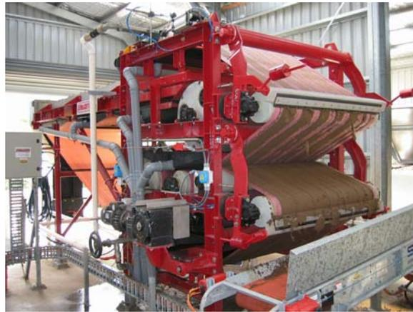
**Figure 1:** *A large belt filter press in operation*
