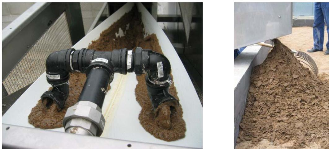
**Figure 4:** Full scale test of the V-fold technology at Picnic Bay MIWR
