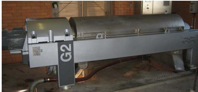
**Figure 2:** *A dewatering centrifuge*
