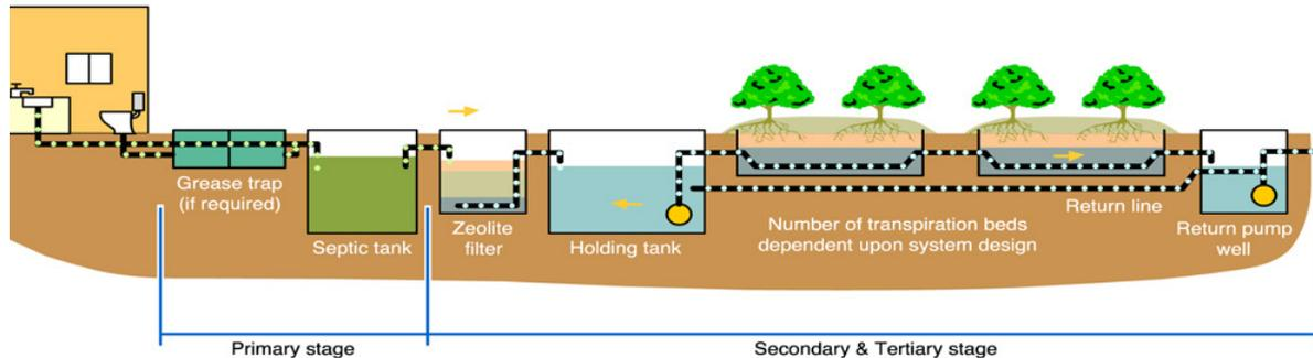
**Figure 1:** *Schematic of KEWT Treatment System*
