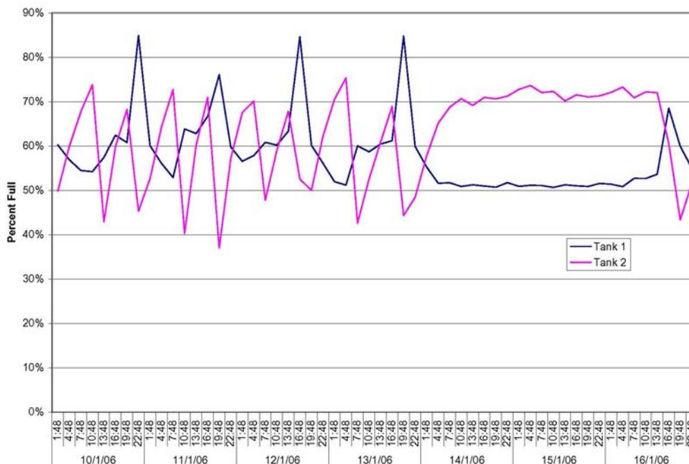
**Figure 3:** Tank Capacity for Child Care Centre KEWT System Over a Week
