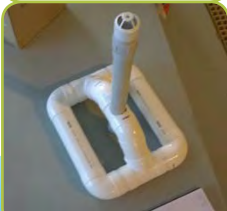
Newly constructed pill dispenser with capacity of 8 chlorine pills
