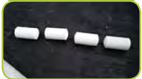
Chlorine pills used in dispenser
