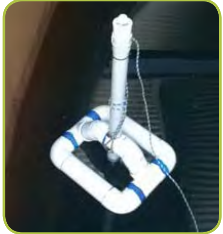
Previous model of pill dispenser (4 pills capacity) now in operation at the Bonny Hills Reservoir
