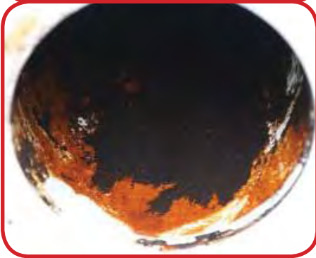
Dislodged particles inside treated water storage tank
